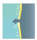
Fleetguard fully formulated coolant can prevent the fatal effect on your engine by creating a protective layer on the liner wall: implosions now take place on this layer and spare the liner surface.
