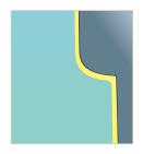
Protective layer created by Fleetguard fully formulated coolant prevents corrosion and erosion.
